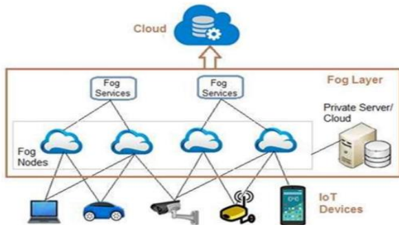
Fig. 2. Architecture of Fog Computing
