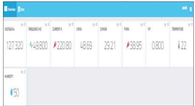
Figure 8: Reading of voltage on Cayenne platform
