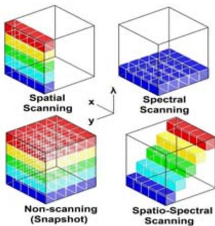
Fig. 4 Technologies for Hyperspectral Data Acquisition[8]
