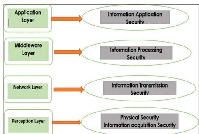
Figure 2: Secured internet of things architecture
