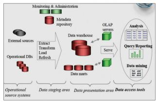
Figure 4: Traditional data warehousing architecture<sup>[11]</sup>
